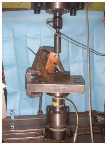
Figure 5. Axial loading of the tibial crest via load applied that is perpendicular to the tibial plateau. The patella was fixed in a rigid split cup connected to the cross-bar of the servohydraulic testing machine and axial load is applied to the tibial tuberosity via the patellar tendon.
