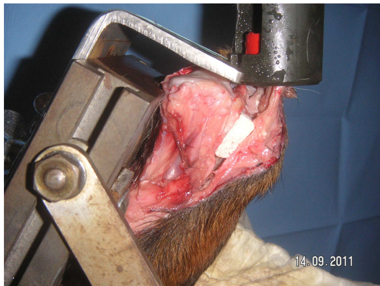
Figure 4. Cyclic testing of the \beta -TCP wedge. The tibial tuberosity is maintained in its position using a block of \beta -TCP.
