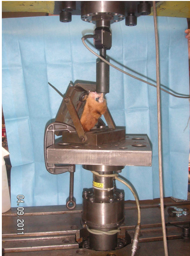
Figure 3. One sample mounted in the materials testing system. The tibia was prepared using a titanium cage to advance the tibial tuberosity (Group 1).
